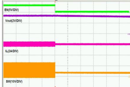
Shutdown Through Enable_no load
